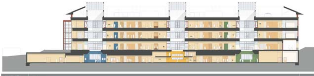
FOUR LARGE ATRIA (THREE SHOWN) FOSTER INTERACTION AMONG BUILDING OCCUPANTS AND CONSERVE ENERGY BY DISTRIBUTING AIR AND LIGHT.
